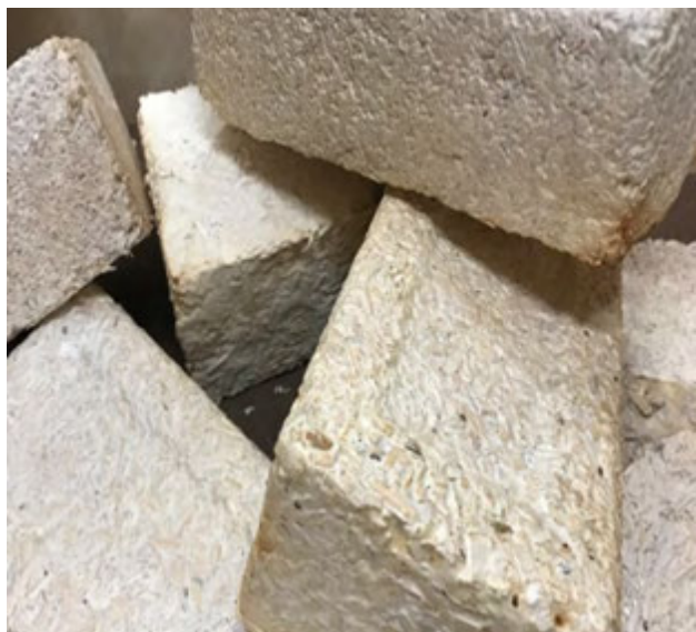
Image: Bricks produced using fungal mycelia, yard waste and wood chips as a part of the Myco-architecture project (Credits: NASA)
