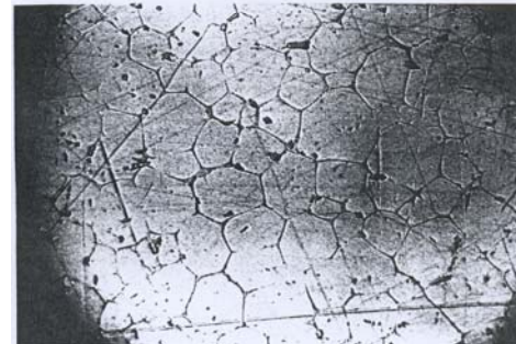
Fig. 3&4: (Average Grain size 22 \mu\text{m} ~ 145 \mu\text{m} ), Magnification: 150 , Micrograph of Al-Mg-Cr alloy work hardened from 3% & 4% under normal static force of 30kN and heat treated at 373 K.
