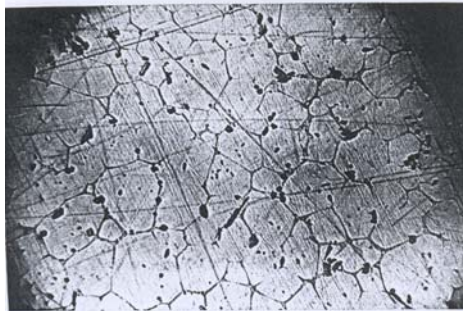
Fig. 5&6: (Average Grain size 20 \mu\text{m} ~ 140 \mu\text{m} ), Magnification: 150 , Micrograph of Al-Mg-Cr alloy work hardened from 5% & 6% under normal static force of 30kN and heat treated at 373 K.
